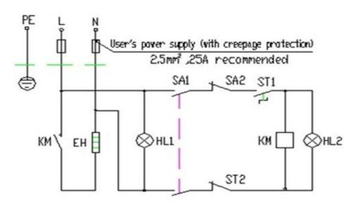
**SA1:Power Switch** SA2:Safe Switch ST1:Temperature Controller ST2:Limit Temperature
