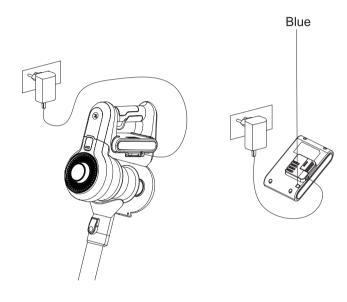
(2) The battery is full while battery pack indicator turns blue.
